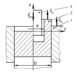
Fig. 1: Inverse extrusion with moving active plate
