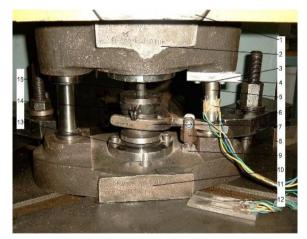
Fig. 3: Assembly for experimental determination of external force requested by the movement of active plate
