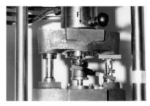
Fig. 2: Die for invers extrusion using active friction forces
