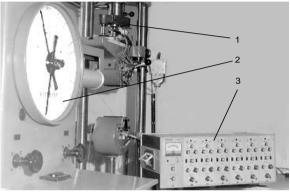
Fig. 4: Stand for experimental determination of forces requested by inverse extrusion using active friction forces
